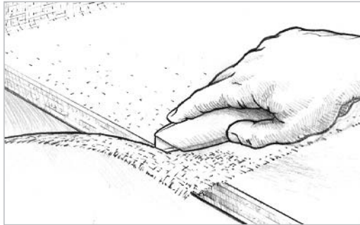
Figure 9-19 Trim excess cloth after the epoxy has begun to gel using a sharp utility knife.
